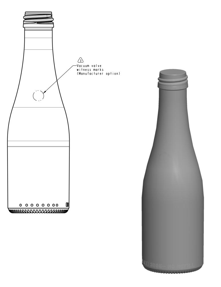
This bottle is based on the current blow and blow design 30636-WS. The process is changing to NNPB. The glass weight has been maintained at 220g.
